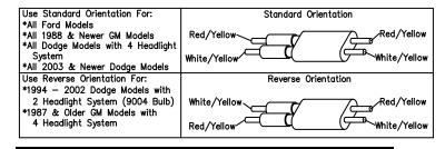
Figure 3. Vehicle Option Connector
