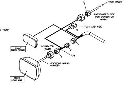
Figure 2. Passenger's Side Single Connections
